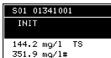
Fig. 3-32 Display during the start phase
