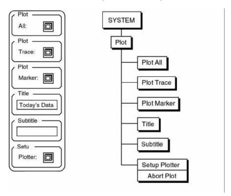
Plot AllThe Plot All key generates a plot of the entire graph, including the scale and<br/>marker information. In single trace display format only the active graph is<br/>plotted. In dual trace mode both traces are plotted. Each feature uses the pen<br/>assigned in the Setup Plotter submenu. The marker is plotted only if it is<br/>presently displayed.Plot TraceThe Plot Trace key plots only the data trace. This allows multiple data traces
