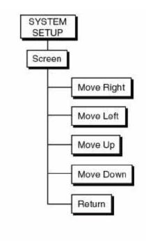
The screen position is stored in non-volatile memory and is retained when the power is turned off. To restore the screen to the default position, power the unit on with the [<-} (backspace) key pressed.
