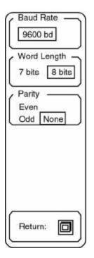
The Setup RS232 key activates the RS232 parameters sub menu. Baud rate, word length, and parity may be configured in this sub menu.
