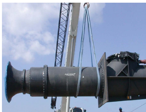
AC-series, Large vertical column pump
