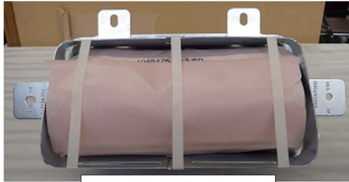
Airbag Reinstallation Complete
