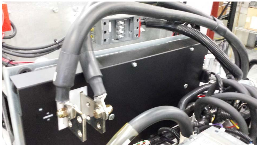
Fig. A-2-1 Connection of Cables
