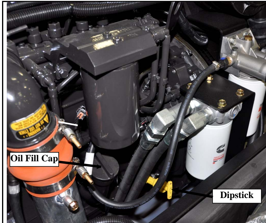
Figure 1-2-2: Oil Fill and Oil Level Check Locations
