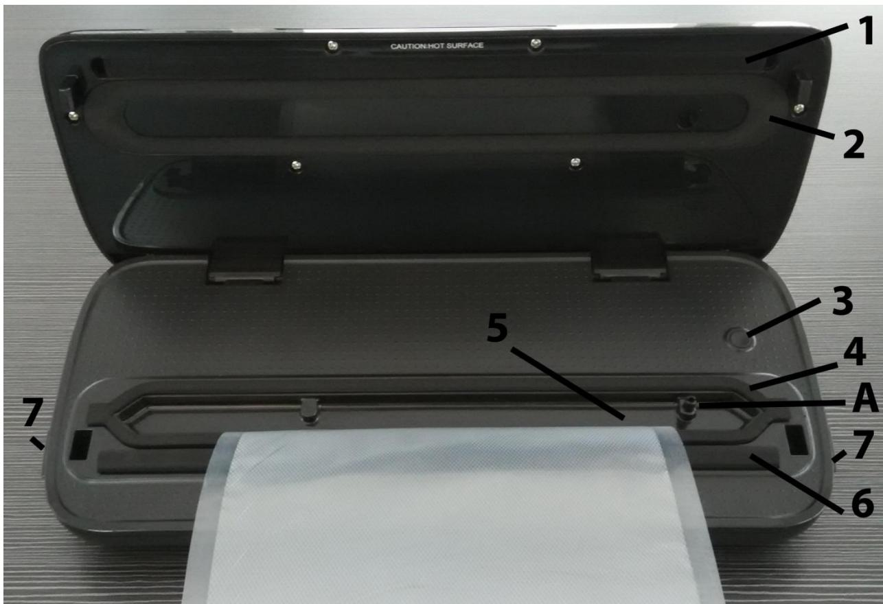
1. Sealing bar- It contains a teflon-coated heating wire. This makes it possible to seal bags without sticking.
