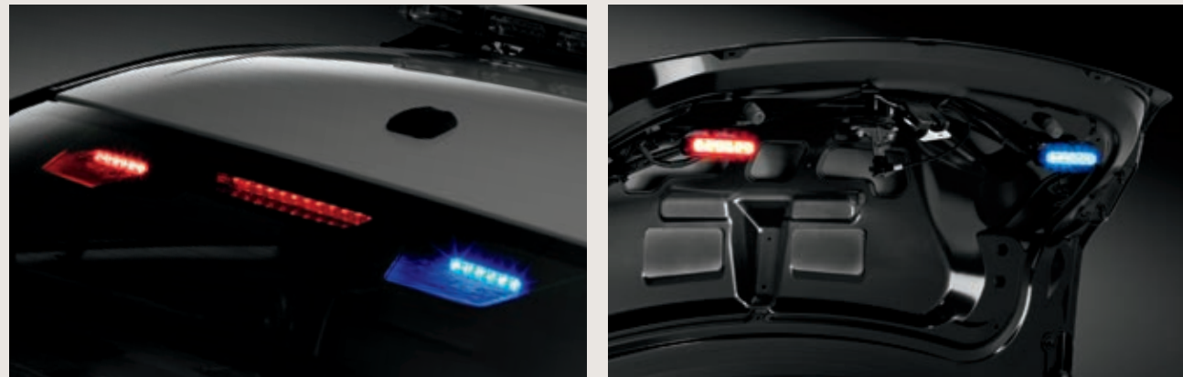
Police back-window lights. Includes (2) backlit flashing, linear high-intensity LED lights (driver side red; passenger side blue) with surround cover mounted inside the back window glass. Police trunk lights. Includes (2) backlit flashing, linear high-intensity LED lights (driver side red; passenger side blue) mounted inside the decklid; lights activate when trunk is open.
