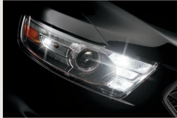
Police headlamp. Includes base headlamp with high-beam wig-wag function and (2) white LED side warning lights.
