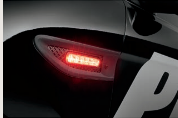
Police side lamps. Fender side markers feature backlit flashing, linear high-intensity LED lamps.
