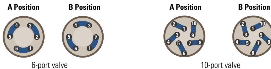
Figure 14. 6-port and 10-port high-pressure valve flow schematics
