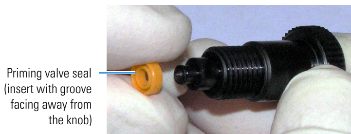
Figure 88. Priming valve and seal
