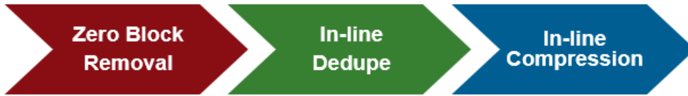
Figure 24: In-line data reduction workflow
