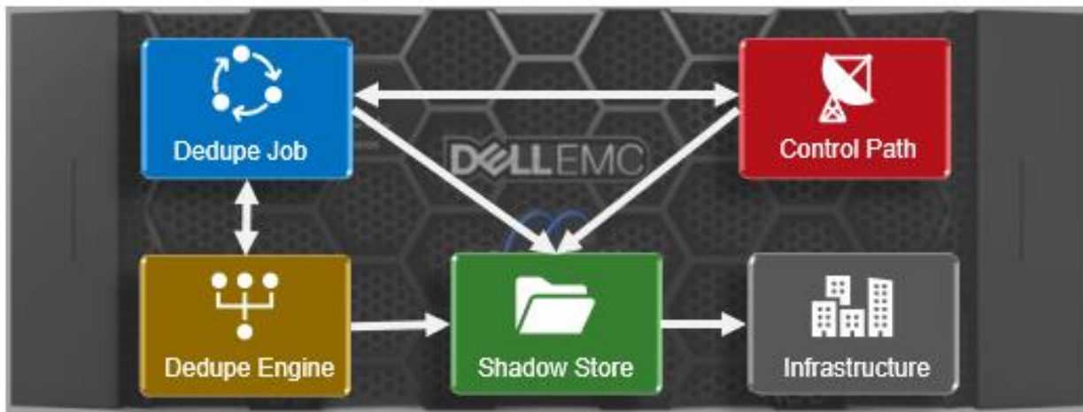
Figure 22: OneFS SmartDedupe Modular Architecture
