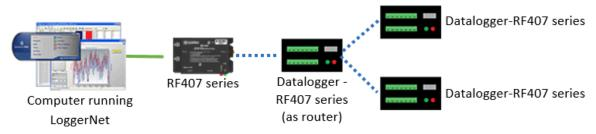
To configure an RF407-series radio to communicate with multiple dataloggers through a router, you must complete the following steps (instruction follows):
