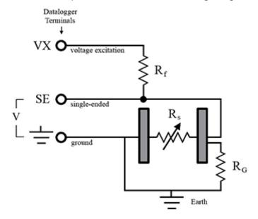
With R<sub>a</sub> in the resistor network, the signal measured from the sensor is described by the following equation:
