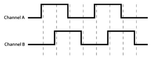
Terminals SE1 and SE2 or C1 and C2 can be configured as digital port pairs to monitor the two sensing channels of an encoder. The ouadrature () instruction can return:
