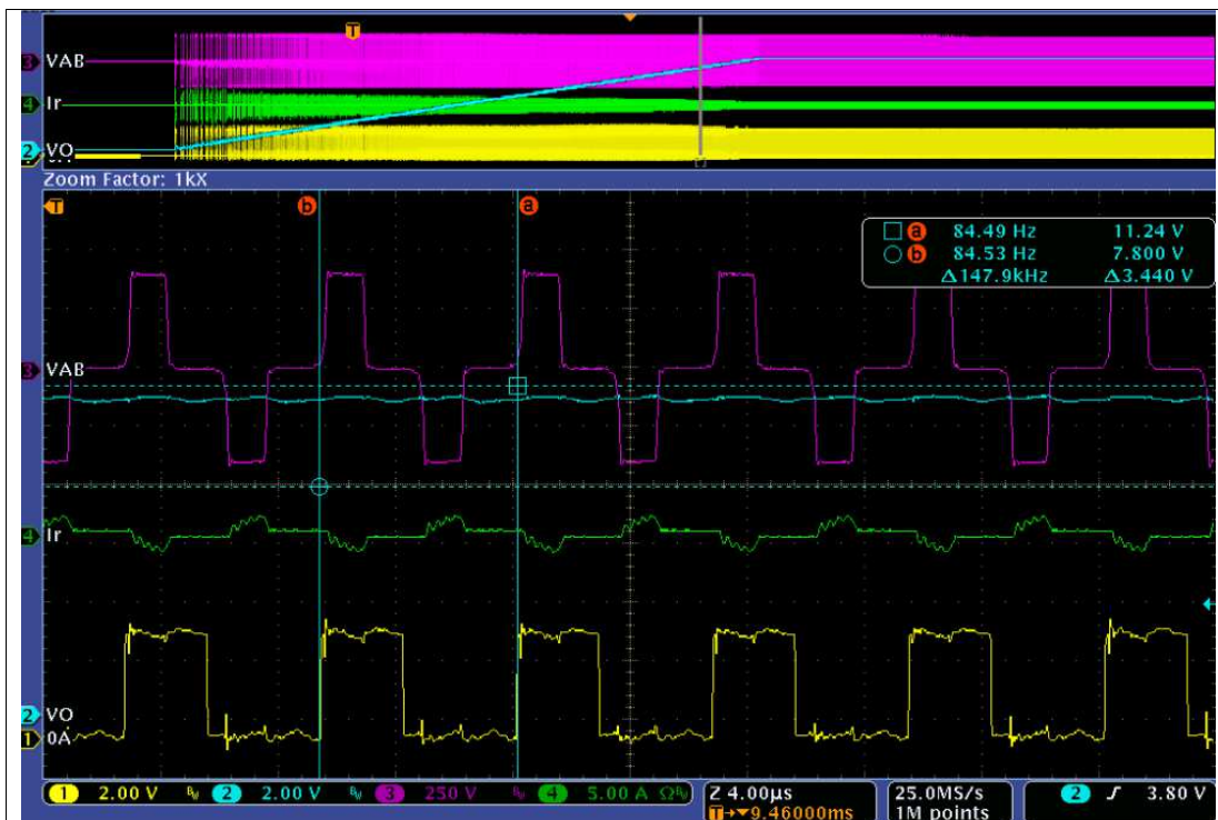
Phase shift mode in low output voltage. V_{in}=380V_{dc} , V_o=12V , I_o=10A Phase angle is increased, switch frequency is 150kHz (maximum switch frequency)
