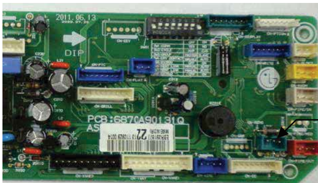
CN-REMO: Remote controller connection
