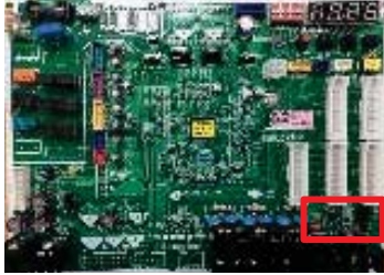
Figure 82: Checking Main PCB (Communication IC).
