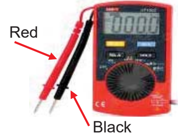
Figure 77: Multi-Meter (Note the Probe Color).
