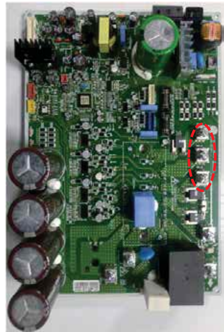
Figure 46: ARUN060GSS4 and ARUB060GSS4 Error No. 22 Compressor Terminal and Wiring Connections.
