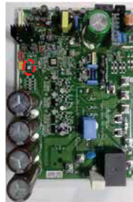
Correct Inverter EEPROM Installation Direction.
