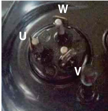
Compressor wiring connections.
