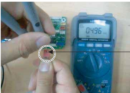
Measure the resistance of outlet pipe temperature sensor.
