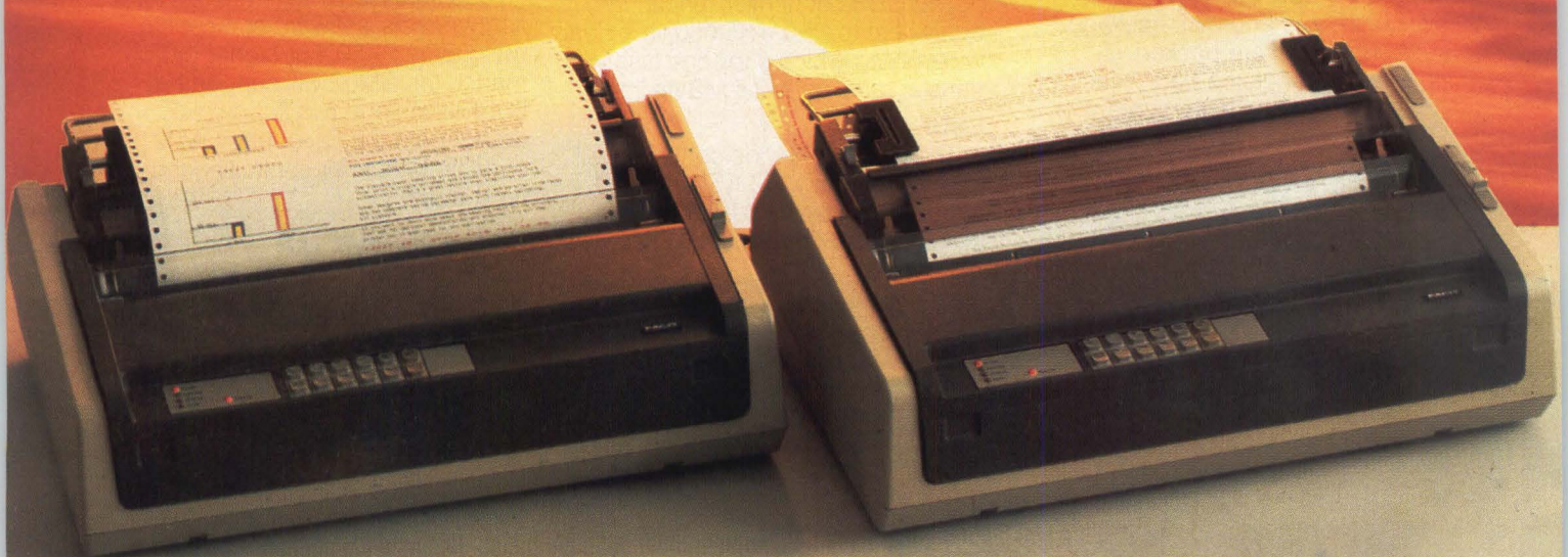
The Facit "C-line" includes the 400 cps, 15-color C7500 and the 250 cps, 7-color C5500
