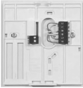
Fig. 2 - Secure Wires to Terminal Strip
