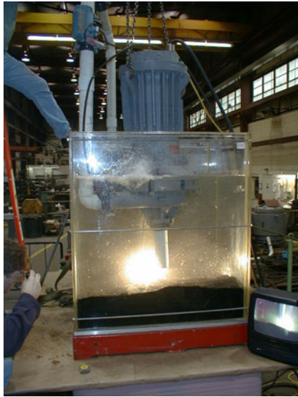
Figure 10 – Pilot Pump Testing Using “Suction Pipe”
