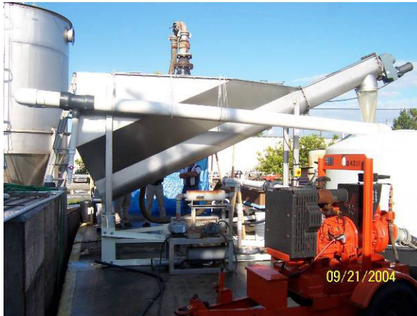
Figure 12 – Grit Classifier Factory Performance Test
