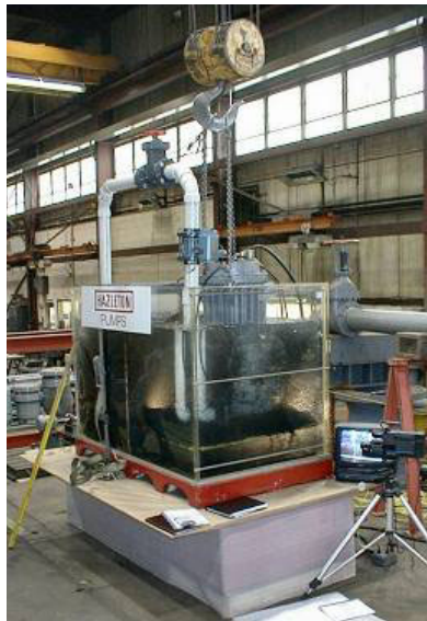
Figure 9 – Pilot Pump Testing Using “Suction Plate”
