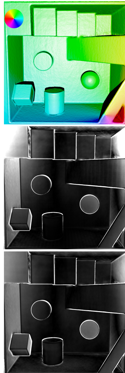
Fig. 7. Left: rendering with optical flow as hsv color overlay; Middle: optical flow endpoint error (0-0.2 pixel, higher errors are white) between ground truth and KinectFusion based scene; Right: stereo disparity error (0-1 pixel, higher errors are white) between ground truth and KinectFusion based scene.
