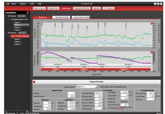
Predict-Pipe: Pipeline Corrosion Results Summary for Wet Gas Internal Corrosion Direct Assessment
