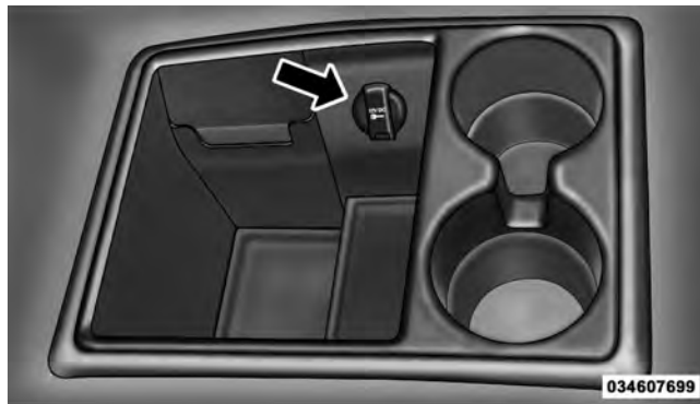
Power Outlet — Floor Storage Bin
