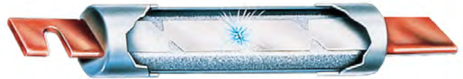
Figure 4: Under sustained overload, a section of the link melts and an arc is established.
