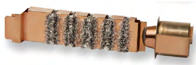
Figure 12: Arc-quenching filler material helps suppress the arcing by melting and forming folgurite.
