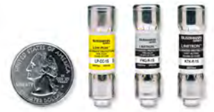
LP-CC, FRO-R, KTK-R — Class CC, 600 V, 200 kA IR up to 30 A
