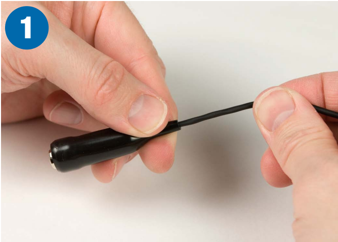
1 Pull the sleeve over the connector so the ends of the connector and sleeve are almost flush.
