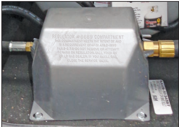
Figure 2-4: LP Gas Regulator
