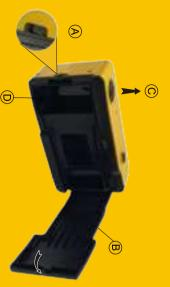
Press the latch (A) in the direction of the arrow and open the camera back door (B) Lift up the film rewind crank (C) and place a new roll of film into the film chamber (D).
