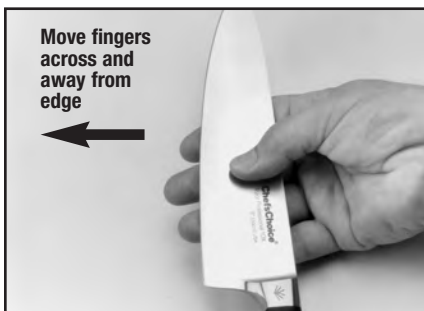
Figure 5. Burr can be detected by sliding fingers across and away from the edge. Caution! See text.
