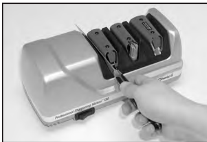
Figure 3. Stage 1. Inserting blade in slot between guide and elastomeric spring. Alternate individual pulls in right and left slots.
