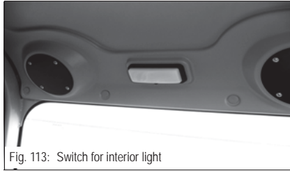
Fig. 113: Switch for interior light
