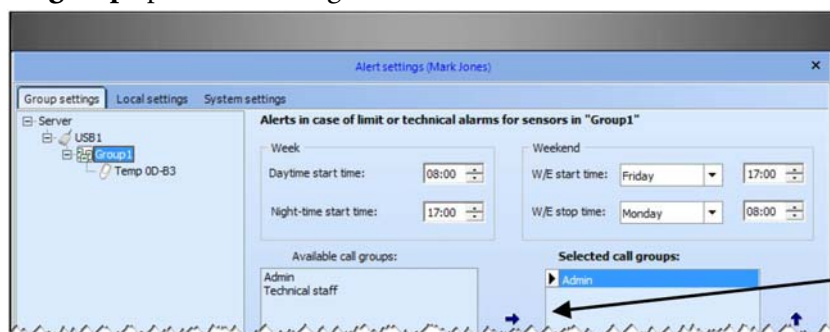
Figure 25. Click on the right arrow (➔) to select call groups to be alerted in case of sensor alarms in the selected group
