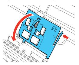
**Caution:** Do not place too much force on the arm inside the cover when replacing the pickup roller.
