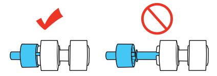
14. Align the notches on the spindle and the scanner, then slide the separation roller into the scanner and gently push it into place. You hear a click when the roller is correctly aligned and locked into place.
