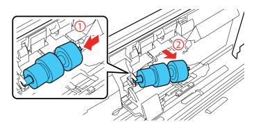
12. Pull the release tab on the separation roller and remove it from the spindle.
