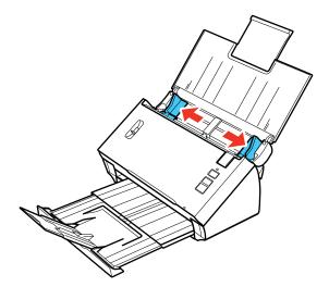
4. Load one plastic card horizontally in the input tray as shown, sliding it in until it meets resistance. Make sure the printed side is facedown and top edge first.
