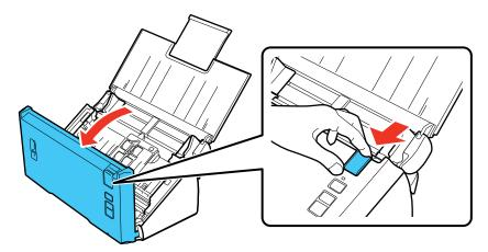
5. Squeeze the tab on the right side of the pickup roller cover and open the cover.
