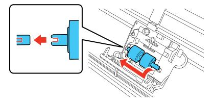
8. To install the new upper pickup roller, align the notches on the roller and slide it to the left. Make sure the smaller roller is on the bottom.
