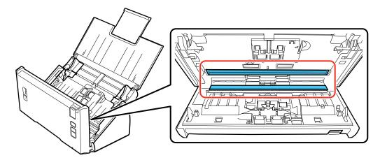
**Note:** If the glass surfaces are stained with grease or some other hard-to-remove material, use a small amount of glass cleaner on a soft cloth to remove it. Wipe off all remaining liquid.
