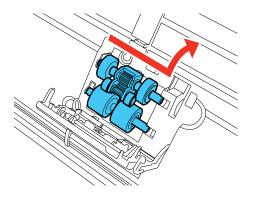
7. To install the new lower pickup roller, align the notches on the roller and slide it to the left.
