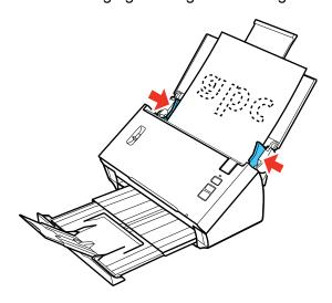
Loading Multiple Sizes of Originals in the Input Tray Original Document Loading Capacity
