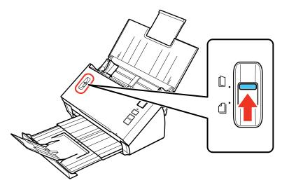
**Note:** To prevent paper jams, make sure to set the separation lever back to its original position when scanning standard single- or multi-page documents.
