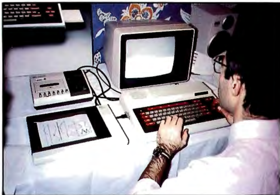
Photo 2: NEC's PC-6000 computer system was introduced recently in Japan and may be brought to this country soon. Shown here is the PC-6001 computer, the Touch Panel graphics tablet, and the data-cassette recorder. The keyboard on the unit shown is of the button type and allows use of an overlay, but NEC is contemplating the use of a keyboard similar to the one used on the PC-8001 before the PC-6001 is introduced into this country. The Touch Panel, expected to sell here for less than $200, would mark a breakthrough in low-cost graphic input devices.
