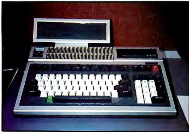
Photo 4: Toshiba surprised everyone when it previewed the T100 at the show. Shown here with the optional flat liquid-crystal display, the T100 is Z80-based and contains 64K bytes of user memory, 32K bytes of ROM, 16K bytes of video RAM, and provision for 32K-byte RAM and ROM packs. Toshiba will be offering Wordstar, dBase II, and all of the Structured Systems Group software, as well as CP/M, when the unit is officially introduced at next month's National Computer Conference in Houston.
