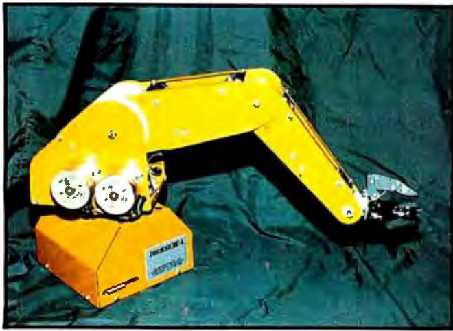
Photo 6: The Armdroid has a maximum reach of 19 inches from the shoulder base.
