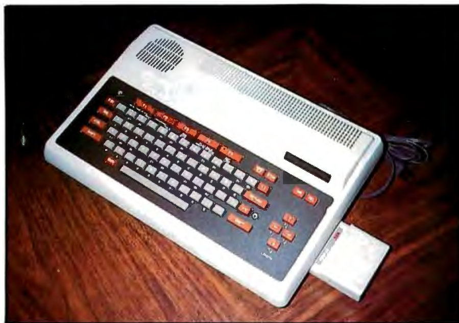
Photo 3: A close-up view of the PC-6001 as shown at NEC's suite at the Riviera Hotel in Las Vegas. Though the keyboard is of the button type, the feel was very good and not at all toy-like. The gray area surrounding the keyboard is a removable overlay which is very useful in applications where it is necessary to redefine the keyboard. ROM packs can be inserted in the right side of the case, and the speaker opening is visible at the upper left-hand corner of the case. Both the style and layout of the keyboard may change before introduction of the PC-6001 into this country.
