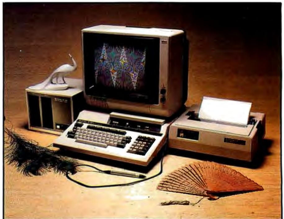
Photo 10: The Hitachi MB-6890 personal computer together with the color video display, double floppy-disk drive, and dot-matrix printer.
