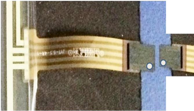
Fig. 9.6: White dots marking correct orientation for connection
