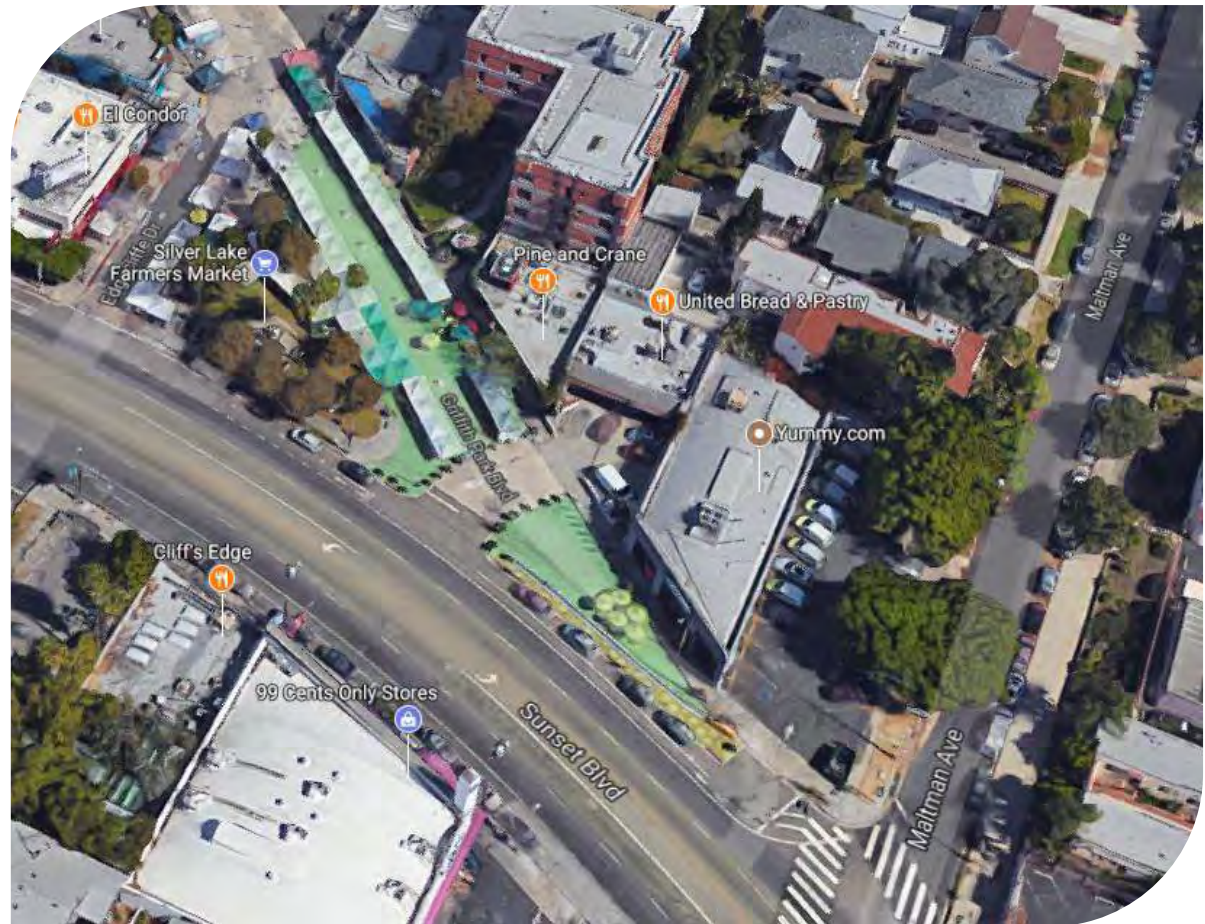
Above: An example of repurposing to remove a skewed intersection (and a redundant link in the roadway network) on Sunset Boulevard in Los Angeles. The resulting space now supports the Silver Lake Farmers Market and increases foot traffic in front of small businesses.
