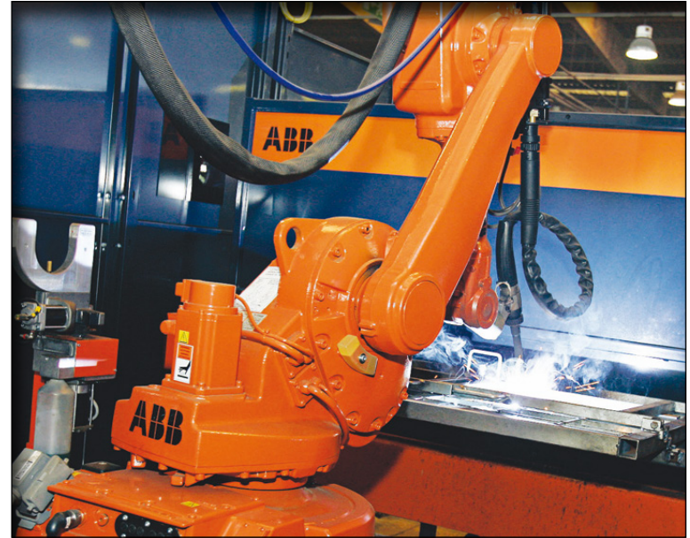
An ABB IRB 1600 robot welds parts in small series production runs for Portuguese company Faramo.
