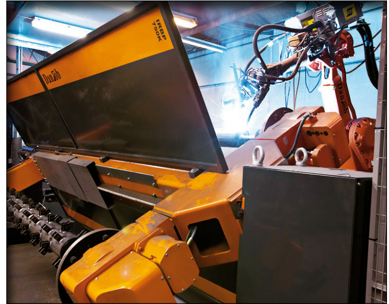
An ABB IRB 2400 robot welds heavy duty agricultural machinery for Danish-based Kverneland Group.
