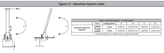
Note: The maximum single span length when using stanchions is 60', see Figure 18. The overall system length can be increased by using intermediate stanchions to create multiple spans in at most 60' increments. For multiple spans two FallTech SteelGrip® Coil Energy Absorbers must be used, see Figure 19.
