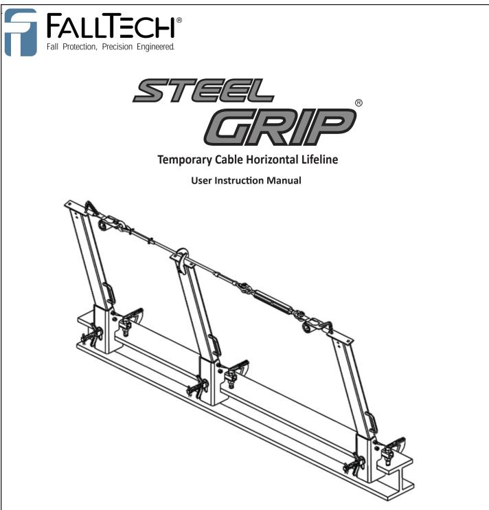
The FallTech SteelGrip<sup>®</sup> Temporary Cable Horizontal Lifeline (HLL) is designed as a temporary reusable anchorage subsystem for the attachment of up to two personal fall arrest systems (PFASs). The FallTech SteelGrip<sup>®</sup> Temporary Cable HLL described in this manual when used as instructed in this manual is OSHA 1910.140 and 1926.502 compliant.
