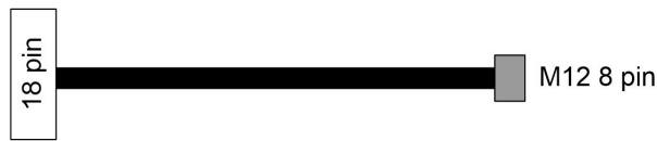
Figure 4 - Pigtail cable: Receiver RX for SG4-N Models (CS-G1-60-B-002)
