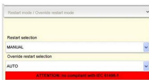
Figure 42 - ACM Configuration: Auto Override Restart Selection
