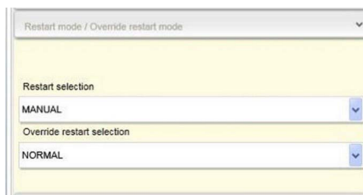
Figure 44 - ACM Configuration: Normal Override Restart Selection
