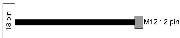
Figure 3 - Pigtail cable: Muting configuration for receiver RX (CS-R1-75-B-002)
