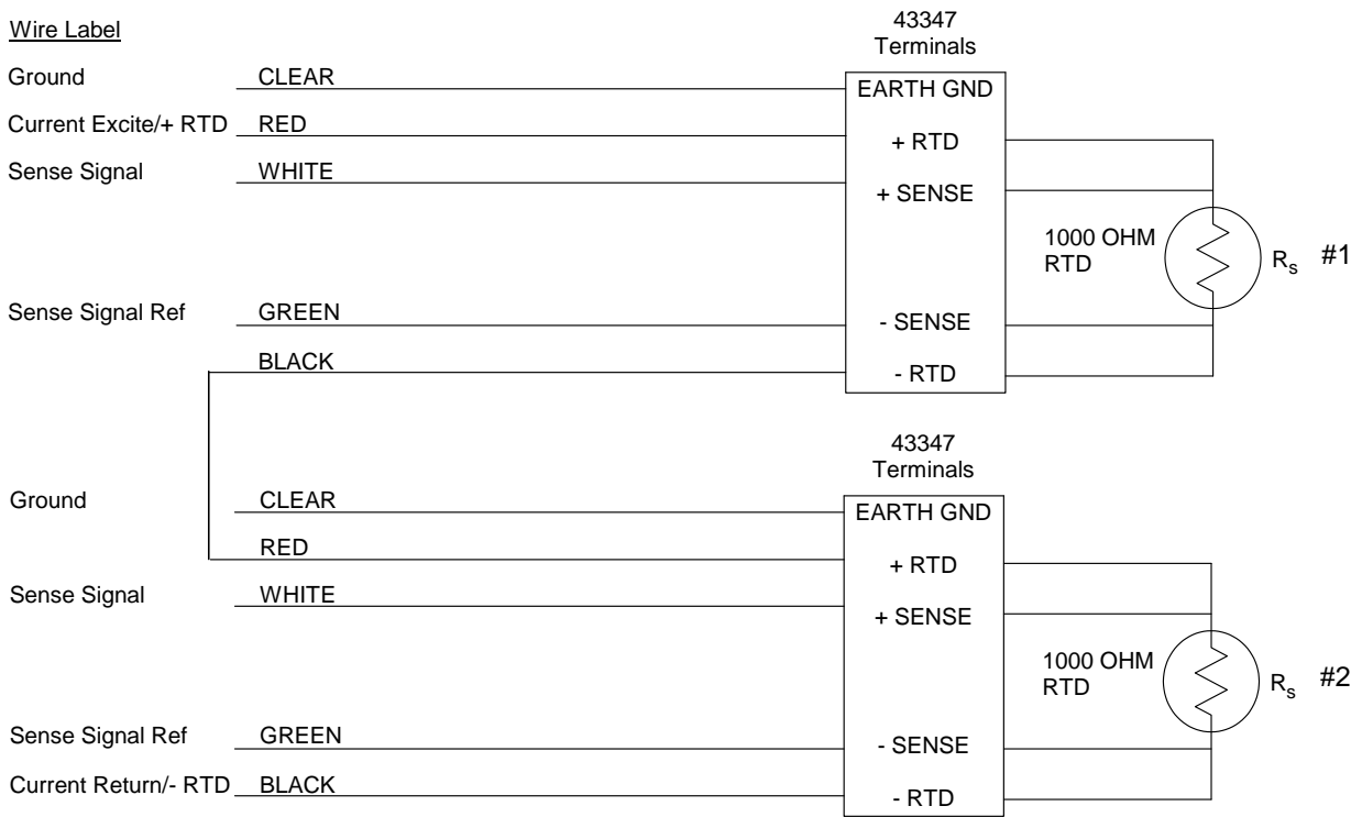
FIGURE E-1. Schematic for two 43347-IX Temperature Probes
