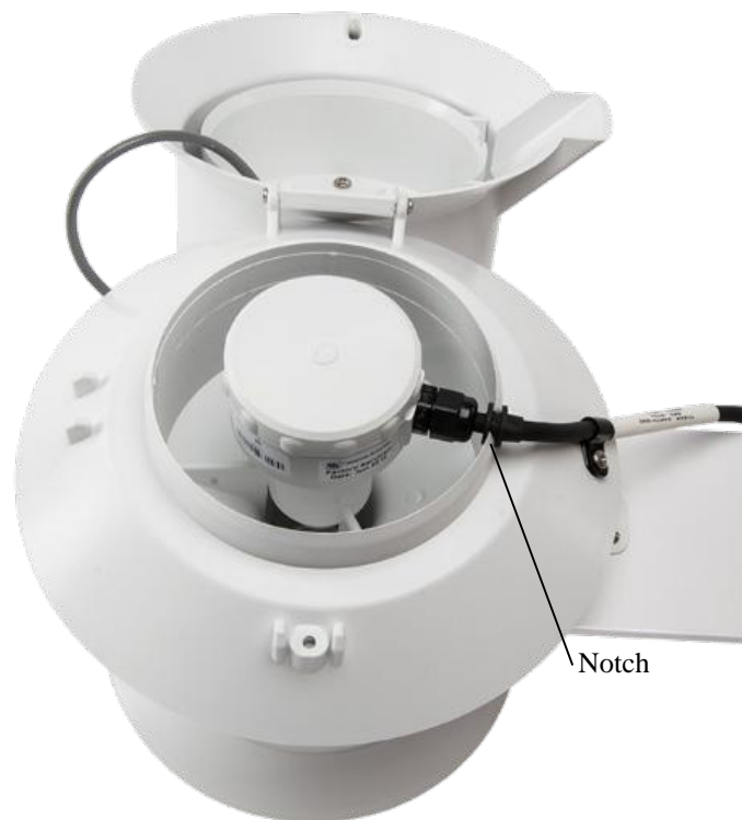
FIGURE 7-4. 43347 probe mounted inside the 43502 shield
