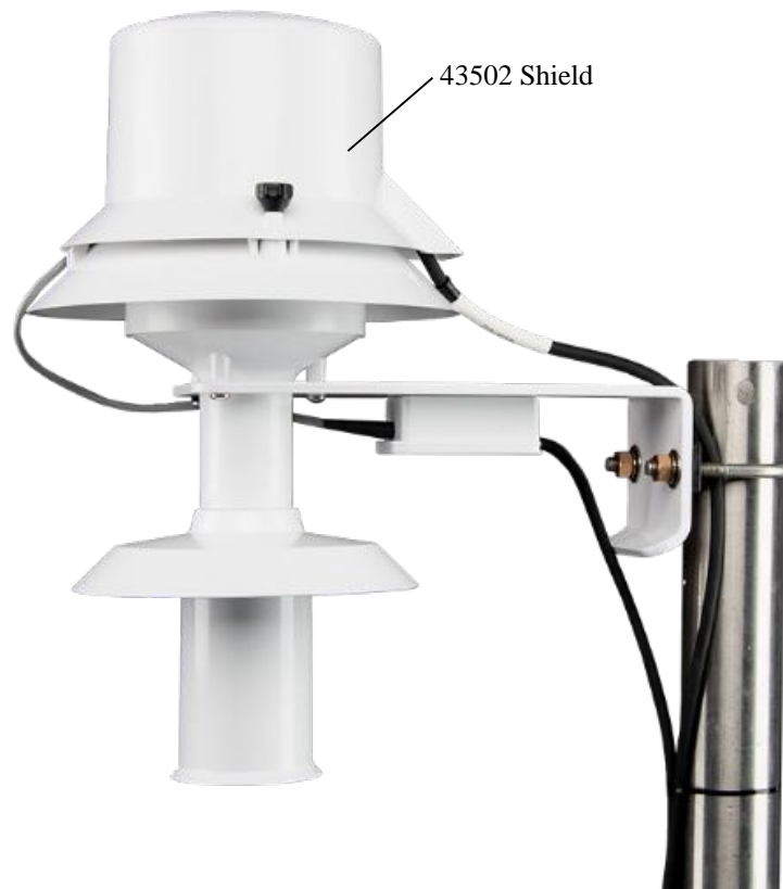
FIGURE 7-1. 43502 Radiation Shield mounted to tripod mast
