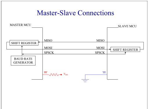
Next, let's look at the SPI master-slave connections. Connect the master MCU to the slave as shown in the figure. Note that before you enable the SPI Modules, you must configure them as a master and slave SPI.
