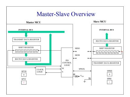
The SPI is built around a double buffered 8-bit shift register with both ends of the shift register brought out to MCU pins. One end of the shift register is connected to the master-in slave-out pin, MISO. This pin acts as an input for the master SPI Module and as an output for the slave SPI Module. The other end of the shift register is connected to MOSI pin.
