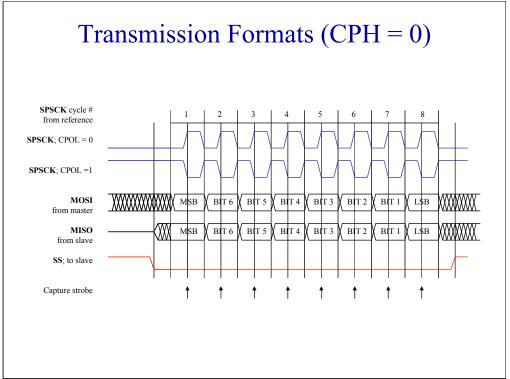
Software can select any of four combinations of the SPI serial clock phase and polarity using the CPOL and CPHA bits. The clock polarity selects an active high or low clock and has no significant effect on the transmission format. The clock phase selects one of two fundamentally different transmission formats. Let's examine SPI transmission for each clock phase, beginning with the clock phase bit set to 0.
