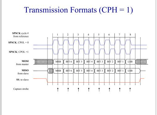
Next, we'll examine SPI transmissions with the clock phase polarity set to 1.
