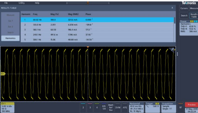
Current harmonics measurements
