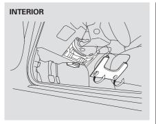
The vehicle's fuses are located in two fuse boxes. The interior fuse box is underneath the steering column. The under-hood fuse box is in the engine compartment next to the battery.
