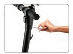
Step 2: Slide the handlebars onto the handlebar stem. Be sure to align all of the screw holes. Then fasten the included screws using the provided allen key tool.
