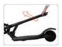
Step 3: Pull the handlebarstem all the way up until it locks in place.
