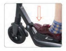
Step 1: Using your foot, press down on the folding buckle.
