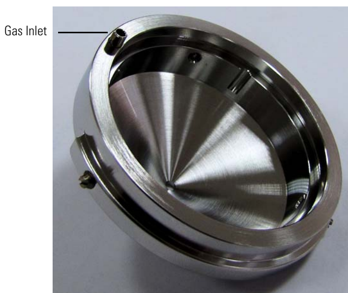
Figure 8-12. Ion sweep cone, showing the gas inlet
