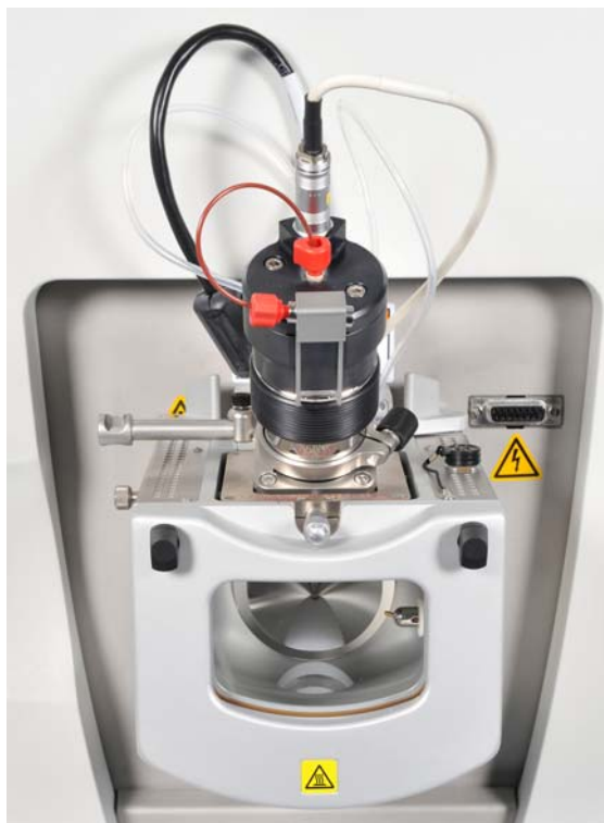
Figure 3-7. Ion Max API source with HESI probe attached
