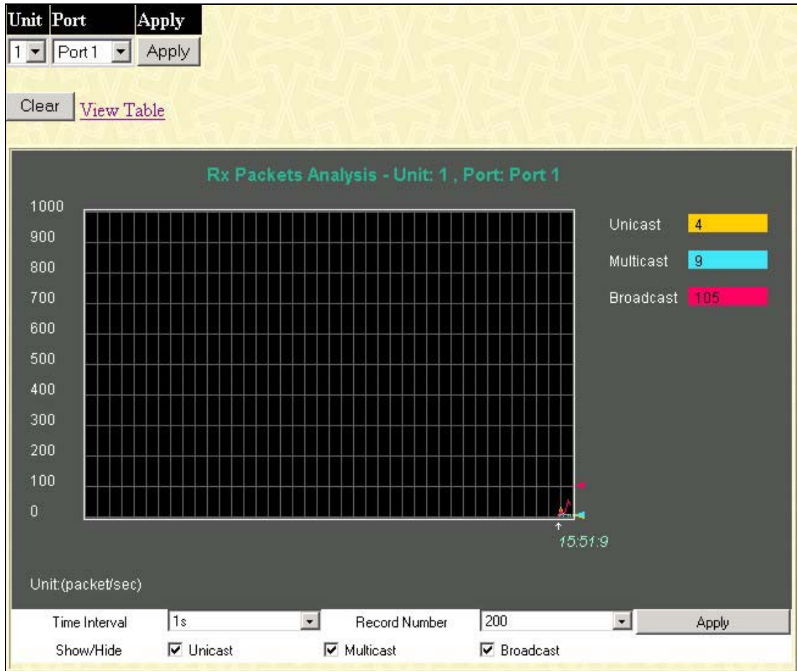
Figure 9- 5. Rx Packets Analysis window (line graph for Unicast, Multicast, and Broadcast Packets)
