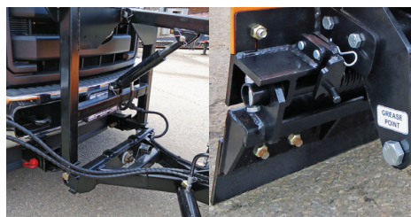
Standard Medium-duty Quick Hitch: for use with MTP & MTP-Flex.
