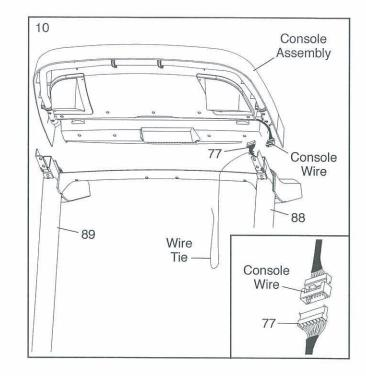
Insert the Upright Wire (not shown) into the Left Handrail (22) as you set the console assembly on the Left and Right Handrails.
