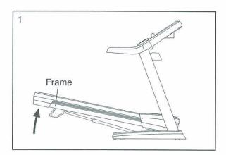
Raise the frame until the latch knob locks in the storage position. CAUTION: Make sure that the latch knob locks.
