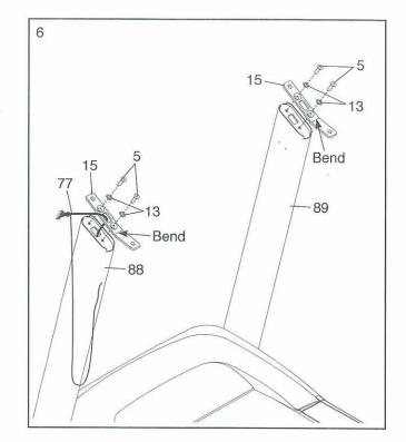
7. Hold the left handrail assembly (B) near the Left Upright (88). Insert the Upright Wire (77) into the large hole in the bottom of the left handrail, and pull it out of the front of the left handrail.
