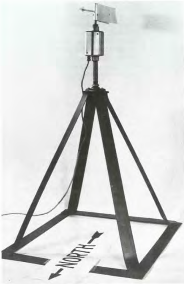
Figure 17.10—Wind vane with marking to assist in true north orientation.
