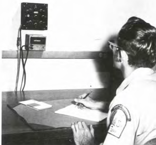
Figure 17.7 —Wind counter and wind direction indicator installed in an office.
