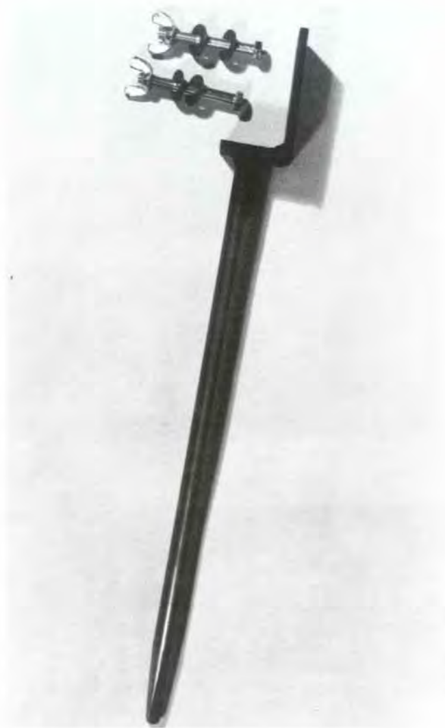
Figure 16.1 —Instrument shelter mounting pin. (See appendix 5 for details.)
