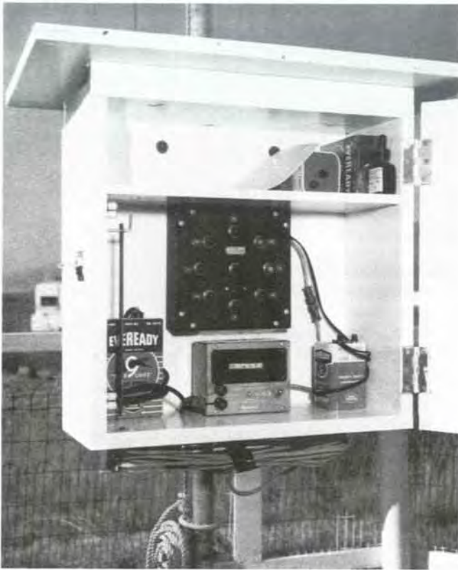
Figure 17.8—Accessory cabinet for on-site installation of wind counter and wind direction readout device. The upper shelf can be used for tools and supplies.
