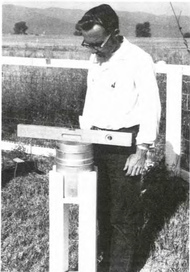
Figure 18.1—The rain gauge installation should be level and plumb.
