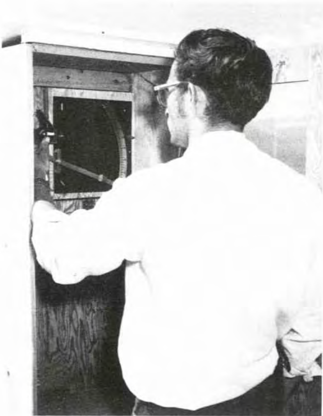
Figure 19.2 —Checking the installation of Forester scale in an Appalachian shelter. Both the shelter and the scale should be level and plumb.
