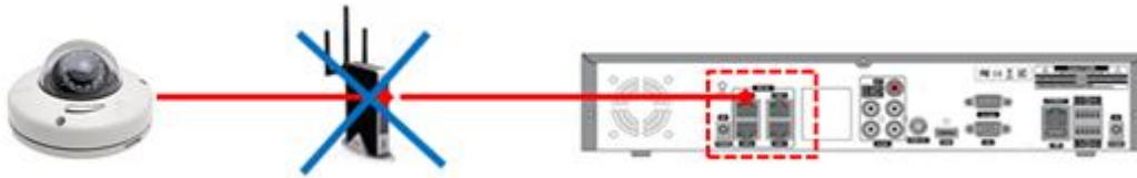
Figure 2.5.2. Incorrect connection with the PoE Ports
