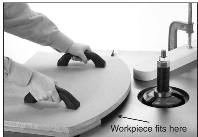
Figure 40. Pattern jig for making curved pieces.
