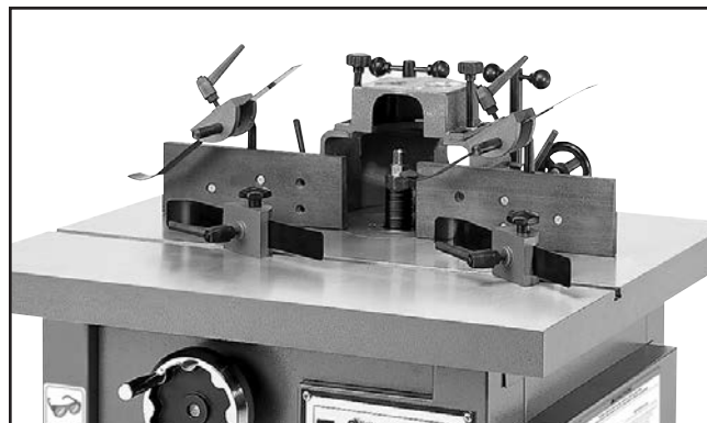
Figure 23. Overview of hold-downs in place.
