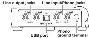
The DS-DAC-10R operates on USB bus power. It does not need an AC adaptor or any other external power supply.
