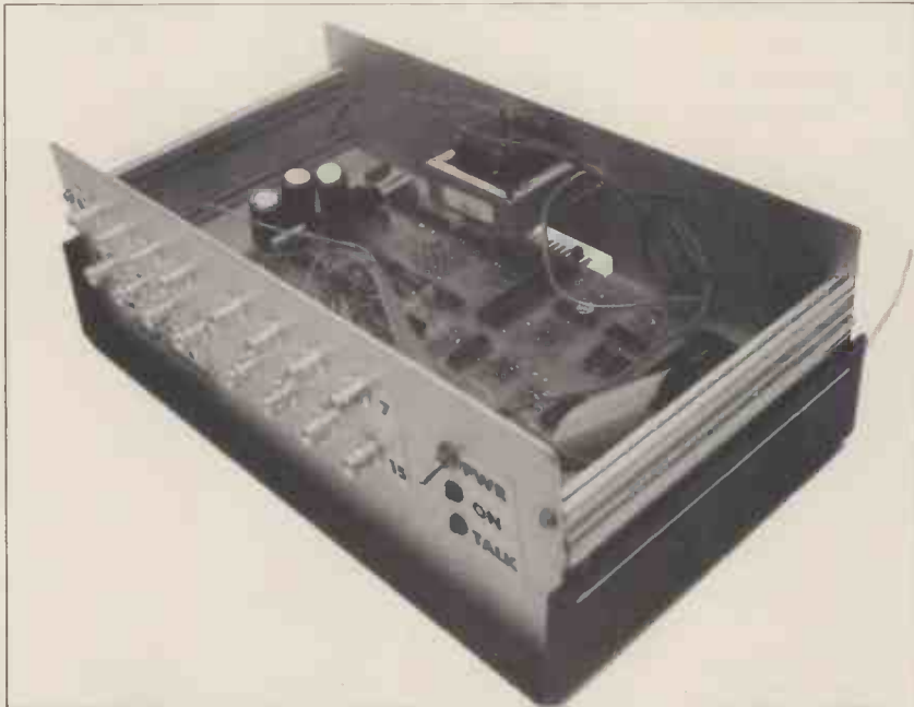
A peep inside a 16-channel analogue to digital converter — typically used to handle signals from devices such as thermometers, pH meters and pressure transducers.
