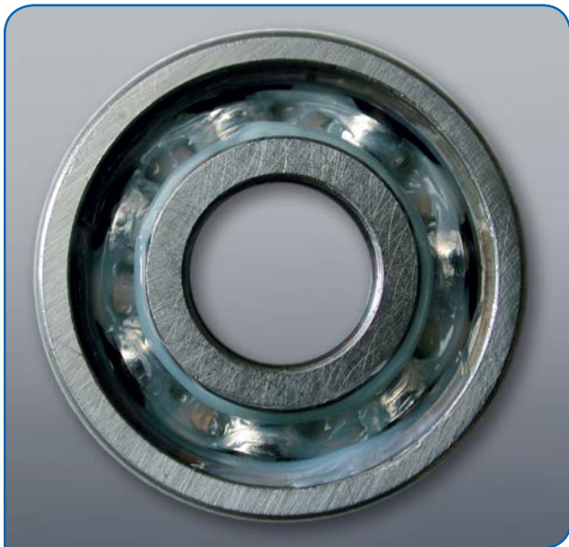
Figure 7 Tips for grease changeover procedures include cleaning grease fittings before lubrication, pumping slowly and applying new grease to a bearing that is turning.
