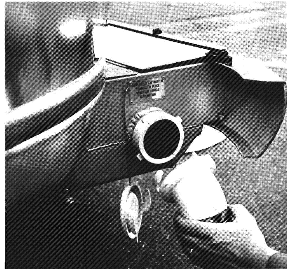
International Rear Bath Sewage Outlet
