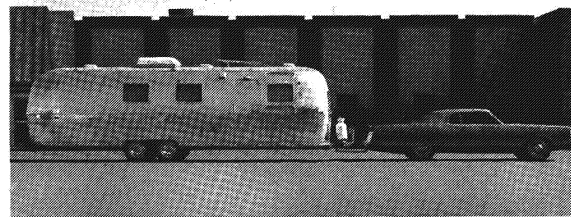
Hitch Installation Proper - Hitch ball level to slightly higher.
