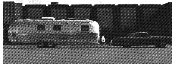
Hitch Low - Load on front wheels too light. Need more tension on load equalizing bars.
