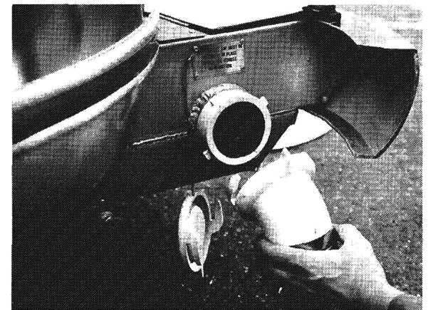
Waste Drain Hose Hook-Up
