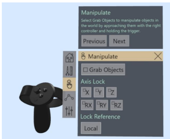
Manipulate tab: Allow objects being grabbed with your hand and limit robot axis while jogging.
