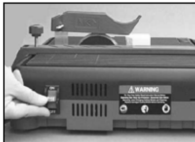
(E) Turn on the MK-145 and verify Cooling Water Flow around Blade Guard.
